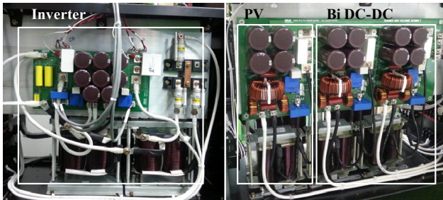
Figure 3. Photograph isolated 10 kW PCS power circuit
