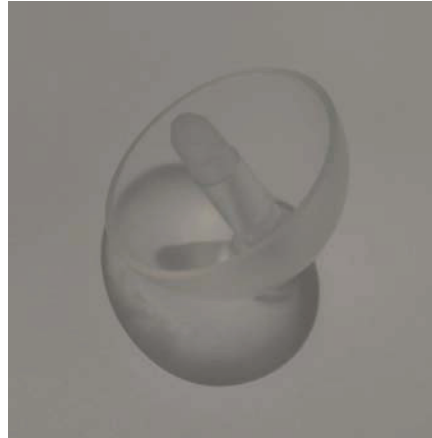
Figure 3 STM's resonator for HRG made from high-purity quartz glass, as a single-piece of 40mm-hemispherical cup and stem through it
