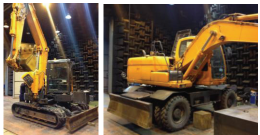
Figure 1 Hydraulic excavators for TPA test
