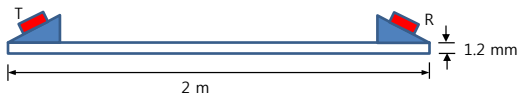
Fig. 1 Experimental set up for A_0 mode Lamb wave generation and reception with variable angle wedge transducers.
