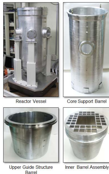
Fig. 1 Manufactured Scale-down Model of APR1400
