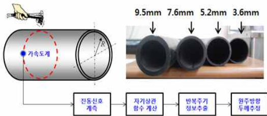
Fig. 1 Experiment for estimating pipe thickness by using measured vibration signal
