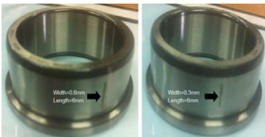
Fig. 4 Seeded defects on the bearing
