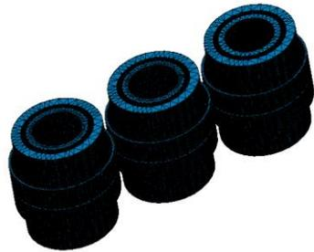
Fig. 1 Finite element model of windings for electromagnetic analysis
