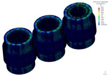
Fig. 2 Distribution of induced electromagnetic forces on the windings.
