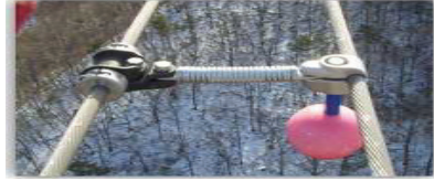
Fig. 5 Target for Vibration Measurement
