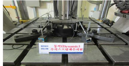
Fig. 7 Spring coefficient experiments
