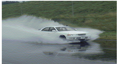
Fig. 1 View of hydroplaning test in proving ground
