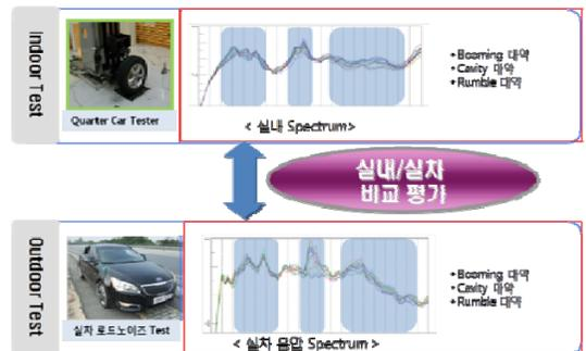
Fig.2 comparison between indoor and outdoor test
