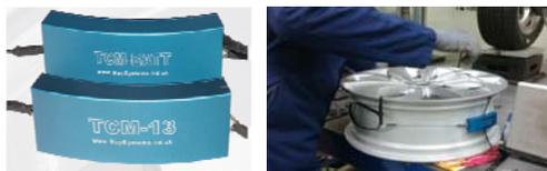
Fig. 4 Tire Cavity Microphone System(TCMS)
