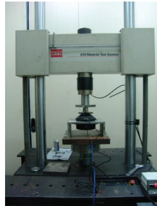
Fig. 2 Experimental Set-up for Measurement of Generated Dynamic Force of Mount
