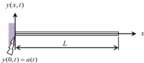
Fig. 2 Cantilever subjected to a support motion
