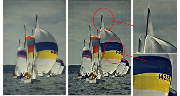
Fig 1. Ringing and blocking artifacts caused by existing method enhancing local contrast. (a) original image and (b) image enhanced by the existing multiband energy scaling method [6] with \lambda = 2 .
