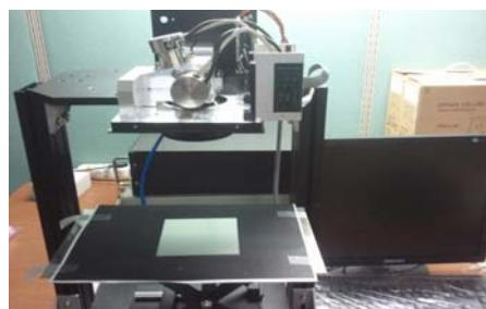
Fig. 1. Experimental setup with fiber laser source
