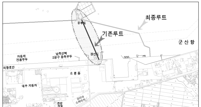
Fig. 3 Altered submarine cable route and location
