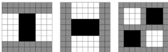
Figure 1 Filter of Approximated Hessian Matrix ( $D_{xx}$ ,  $D_{yy}$ ,  $D_{xy}$ )
