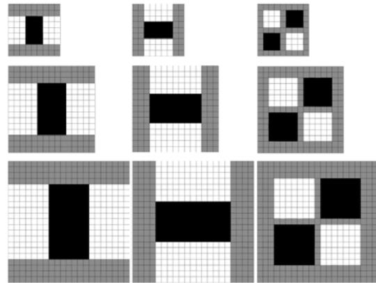
Figure 2 Changes of Scale of Filters ( $D_{xx}$ ,  $D_{yy}$ ,  $D_{xy}$ )
