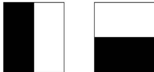
Figure 3 Harr Wavelet Filter (x direction, y direction)
