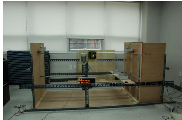
Figure 4. Earth retaining wall test-bed of a ubiquitous environment to collect data
