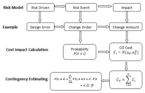
Figure 3 Probabilistic Contingency Calculation Model
