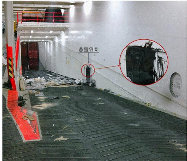
Fig. 2 Damage due to Impact by Trailer and Container
