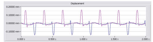
Fig. 5 Displacement signal including shape errors at upper and lower sides
