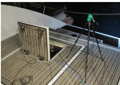
Fig. 8 Microphone position on hull deck
