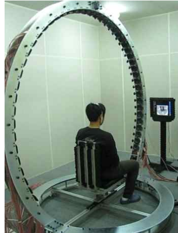
Figure 1 HRTF measuring system
