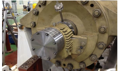
Figure 6 Counterweight for Resonance Reduction
