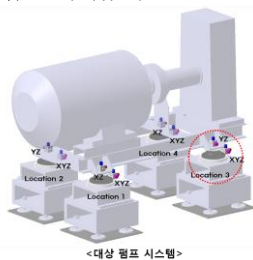
Fig. 4 Objective System Including Mount for Reduction of Transmitted Force to Hull Body
