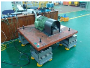
Fig. 4 Objective System Including Mount for Reduction of Transmitted Force to Hull Body
