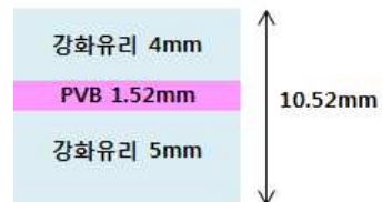
Figure 3 Reference specimen for transmission loss comparison with test specimens
