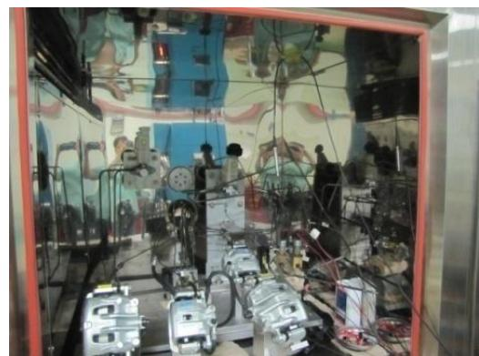
Figure 3 Picture of HILS Chamber
