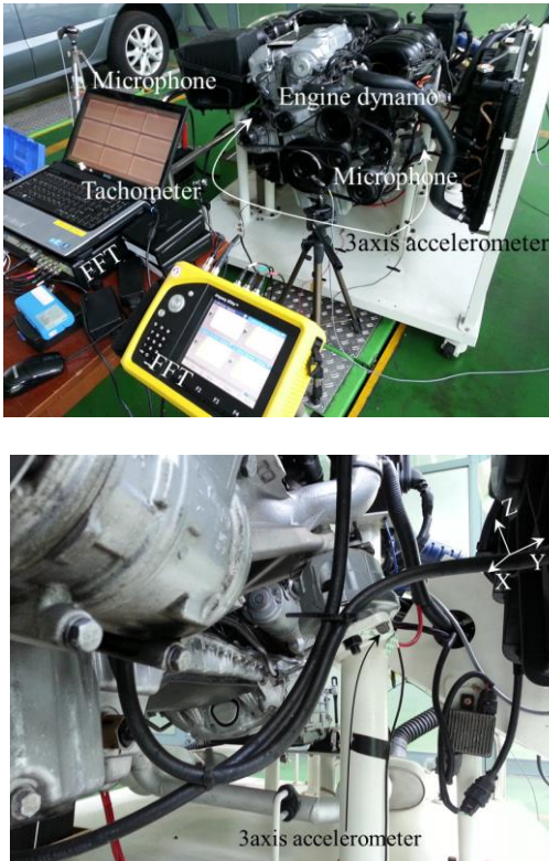
Fig. 2 Noise and vibration measurement of engine dynamo
