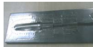
Fig.3 Protective Structure for Strain Gauge of APR1400
