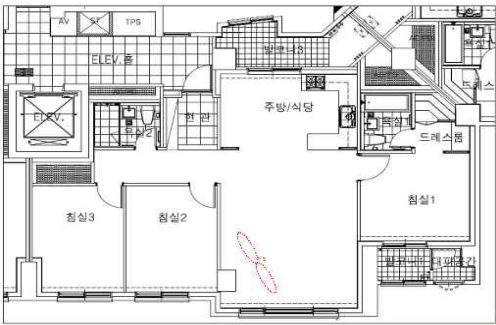
b. Location marked with walking and running Figure 2 plan view of the psycho-acoustic experiment and Position of floor impact source
