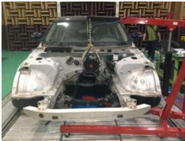
Fig.9 Experimental setup to get transfer function of trimmed body
