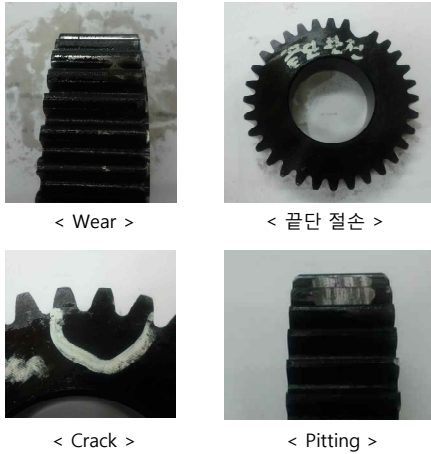
Figure 2 Damaged gear box for experiment
