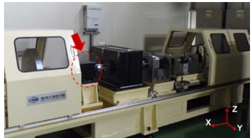
Figure 1 An experimental mock-up model and measurement position (in the red dotted circle)
