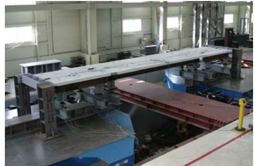
Figure 3 3 spans girder bridge test
