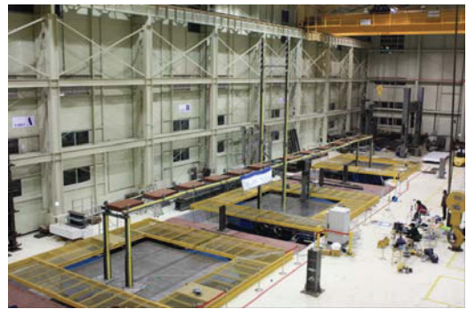
Figure 2 2 spans cable-stayed bridge test
