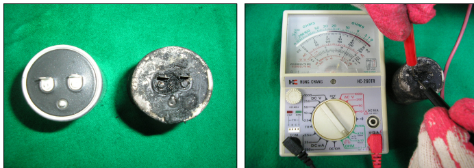
(a) normal and damaged capacitor (b) The damaged capacitor
