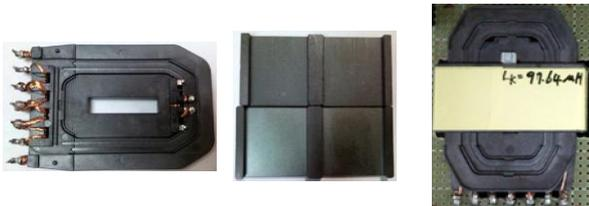
(a) Assembly of Bobbin (b) EE Core (c) Transformer
