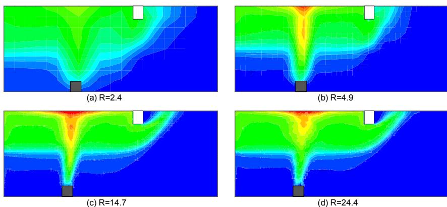
Figure 1. Comparison of time averaged temperature field during the quasi-steady state for 511 kW fire.
