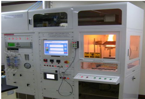
Fig. 1. Schematic diagram of cone calorimeter
