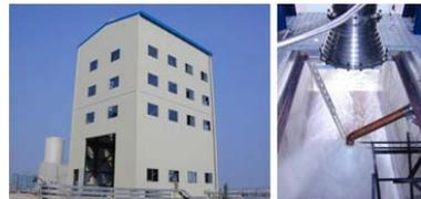
Fig. 6 Flame Deflector in PTA-II Test Stand of KSR-III
