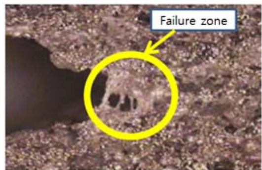
Fig. 2 Failure zone of a highly filled elastomer
