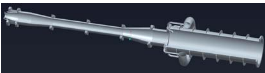
Fig 6. Sub-scale Supersonic Diffuser Firing Test Rig
