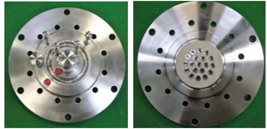
Fig. 4 Mixing Head of Sub-scale Thrust Chamber
