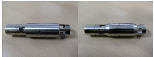
Fig. 5 Design modification on the spool end tips (Left : before modification, Right : after modification)
