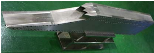
(a) External View of the Mach 5 Scramjet Model
