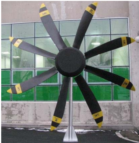
Fig. 8 View of prototype propeller assembly with 8 blades
