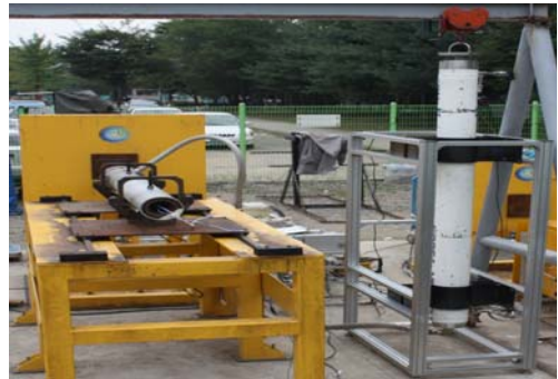
Fig. 2 Oxidizer Tank & Hybrid Rocket motor configuration
