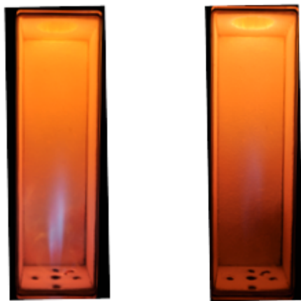
Conventional flame Flameless combustion Fig. 1 Comparison of conventional flame and flameless combustion
