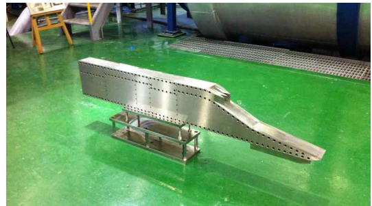
Fig. 5 Hydrocarbon-fueled scramjet engine (C1 model)
