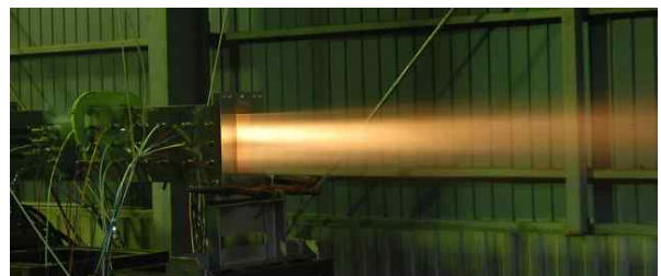
Fig. 2 Scramjet Engine Combustor Test
