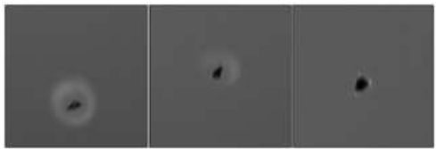
Fig. 5. Ignition of char particle, coal A, 150-200 \mu m
